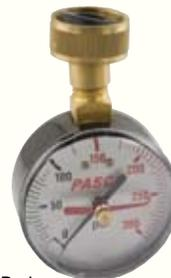
Excellent to determine if P/T valve is leaking from failure or if leaking is caused by surge or excessive pressures. (Attach gauge to Boiler Drain Valve overnight.) LAZY hand operates over entire gauge range of 0-300 psi.
