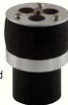
To prevent basement flooding flood-guard operates like a check valve to seal off water back-up caused by overloaded sewers. Water flows normally through the drain until the sewer begins to back-up. Then the flood-guard float rises to seal off the drain opening until the water recedes.
