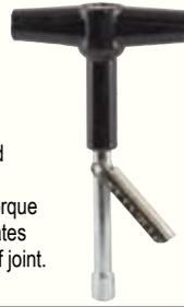
For assembling no-hub soil pipe couplings. Preset 60 inch pound torque. 5/16" hex socket grips securely "clicks" when proper torque has been developed and eliminates guesswork to obtain a leak-proof joint. Handy reversing lever.
