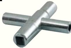
For stopcocks, sillcocks and valves, used when handles have been removed. Fits 1/4", 9/32", 5/16" and 11/32" square stems. High quality steel, case hardened and zinc plated.
